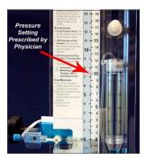
Once the pressure transducer has been "zeroed," the drip chamber needs to be adjusted back to its original setting.
