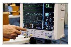
• The clinician then pushes the zero button on the bedside monitor and the transducer is now "zeroed" to atmospheric pressure
